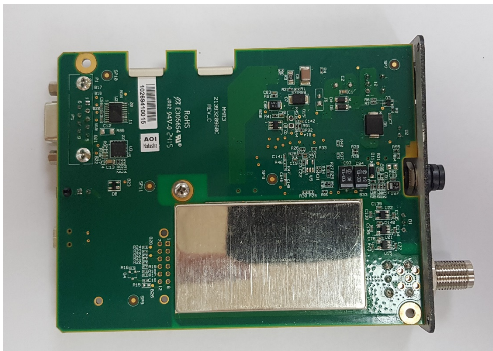
PCB bottom with RF shield
