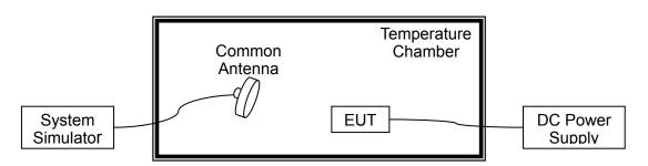
The EUT, which is powered by the DC Power Supply directly, is located in the Temperature Chamber. The EUT is commanded by the System Simulator (SS) to operate at the maximum output power i.e. Power Control Level (PCL) = 5 and Power Class = 4. A call is established between the EUT and the SS via a Common Antenna.
