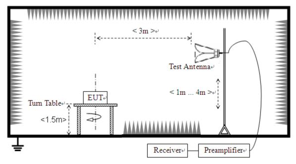
The EUT is located in a 3m Full-Anechoic Chamber, the cable loss, air loss and so on of the site as factors are pre-calibrated using the "Substitution" method, and calculated to correct the reading.
