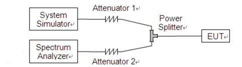
The EUT is coupled to the Spectrum Analyzer (SA) and the System Simulator (SS) with Attenuators through the Power Splitter; the RF load attached to the EUT antenna terminal is 500hm; the path loss as the factor is calibrated to correct the reading. The EUT is commanded by the SS to operate at the maximum output power i.e. Power Control Level (PCL) = 5 and Power Class = 4. A call is established between the EUT and the SS.
