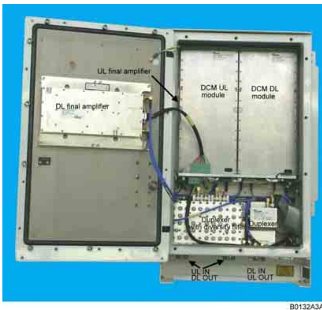
figure 5-3 RF path of a Node C, exemplary
