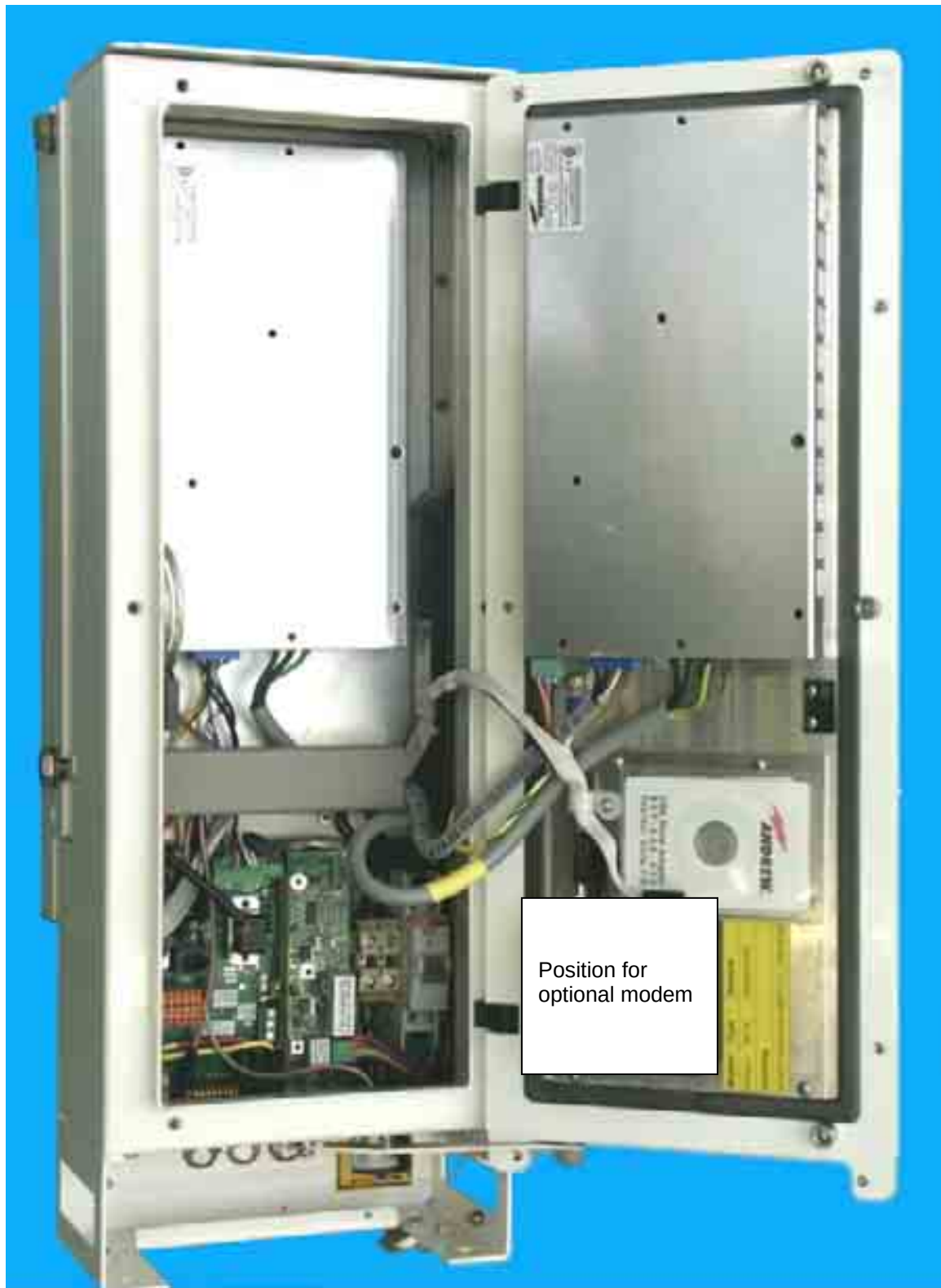
figure 7-5 Layout of the Interface Unit, exemplary
