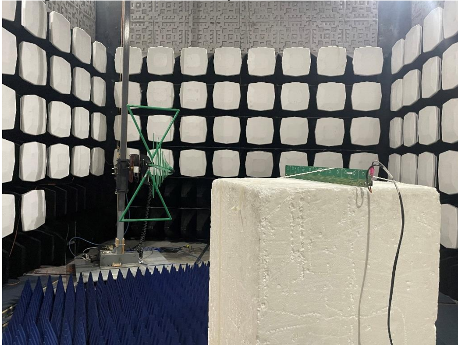
Figure 5.2-Reference test setup of an antenna – Y- Orientation
