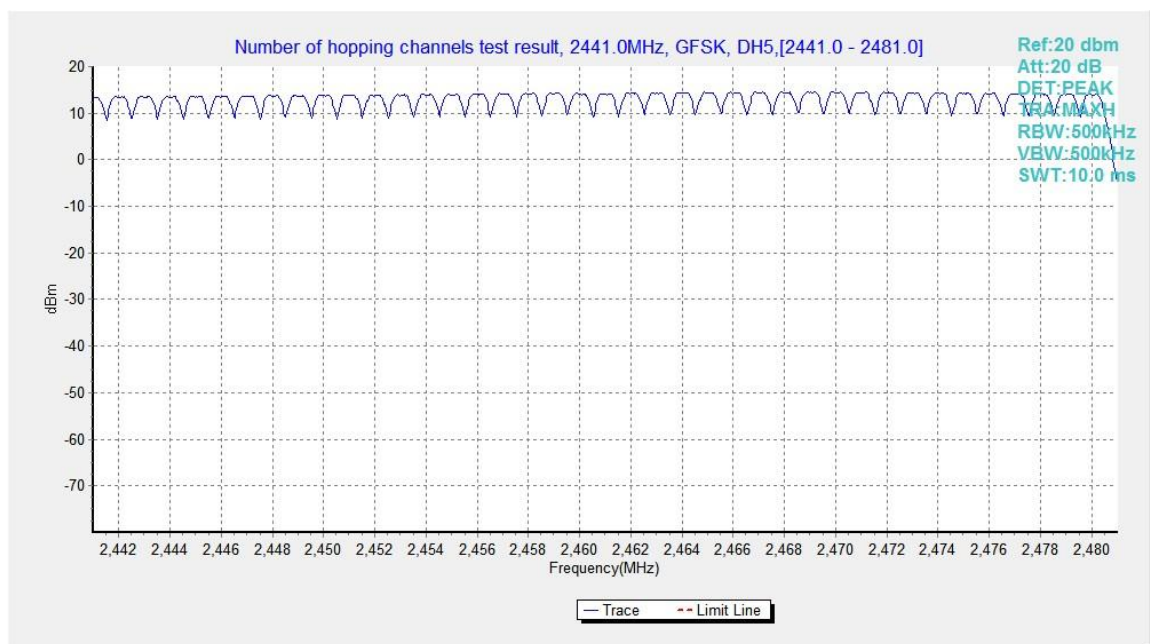
Fig.95. Number of hopping frequencies: GFSK, Channel 40 - 78
