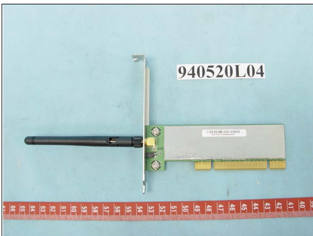
Dipole antenna with 2.00dBi gain
