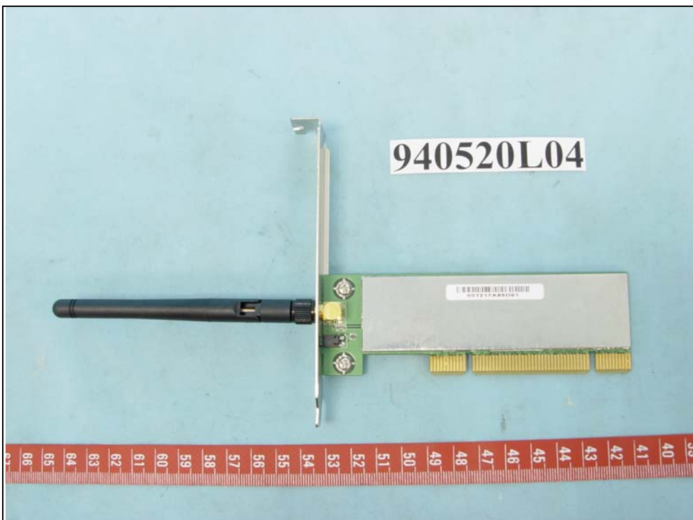
Dipole antenna with 2.48dBi gain
