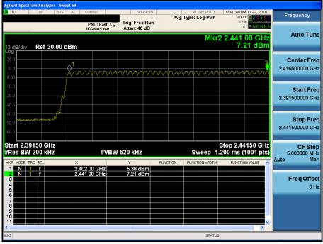
Number of Hopping Frequencies 2(FH) <u>Hopping mode : Enable &  $\pi/4$ -DQPSK</u>
