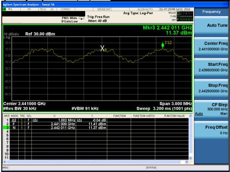
Carrier Frequency Separation (FH) <u>Hopping mode : Enable & π/4-DQPSK</u>
