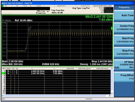
Number of Hopping Frequencies 2(FH) <u>Hopping mode : Enable & GFSK</u>
