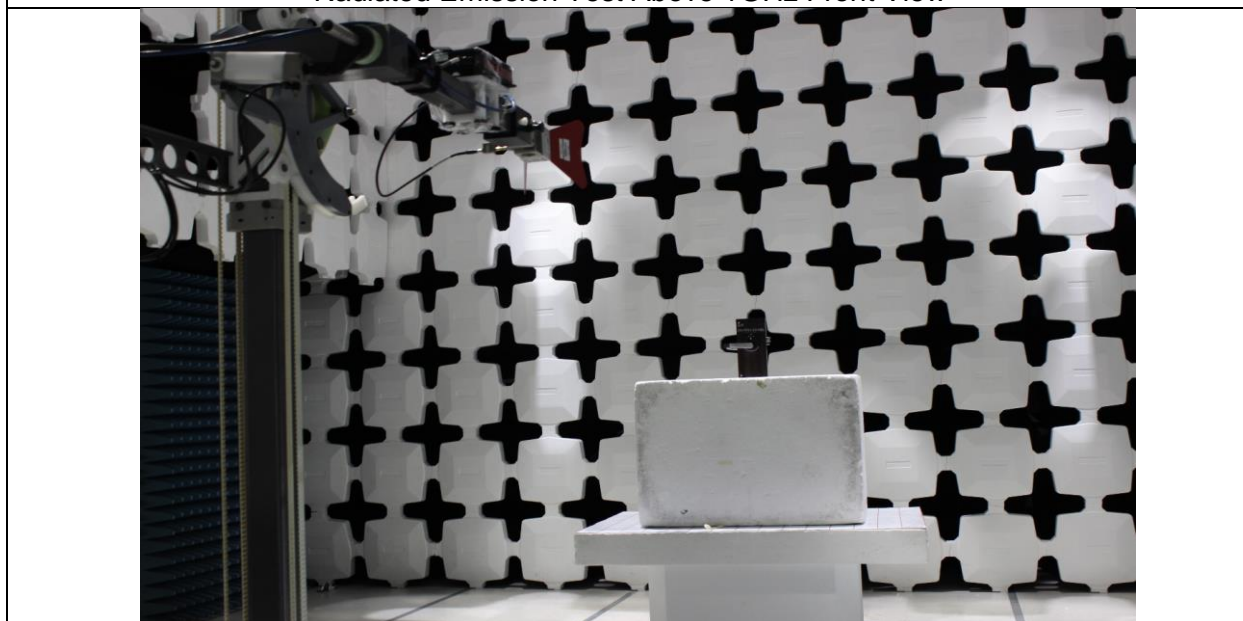
Radiated Emission Test Above 1GHz Rear View
