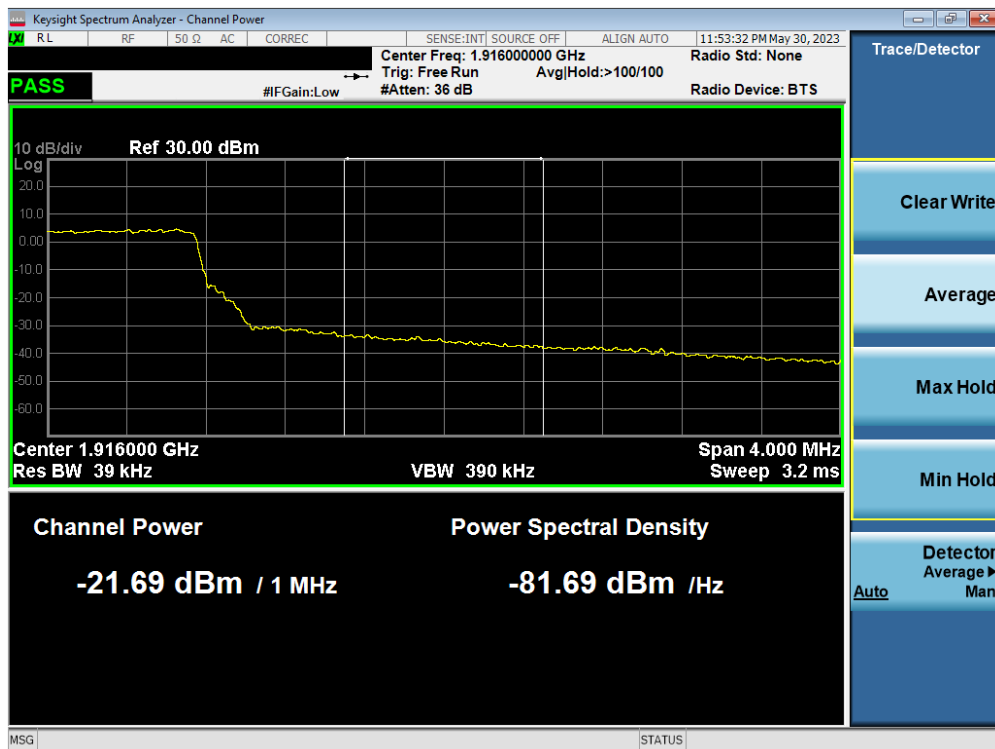
Plot 7-43. Extended Upper Band Edge Plot (LTE Band 25 – 5MHz QPSK – Full RB Configuration)
