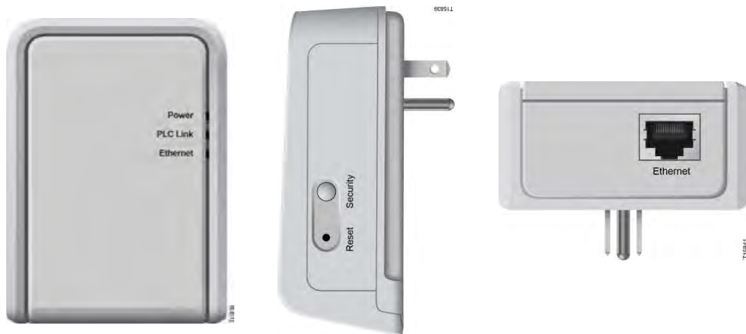
Figure 31: IP522CG – Front, Side and Bottom Panels
