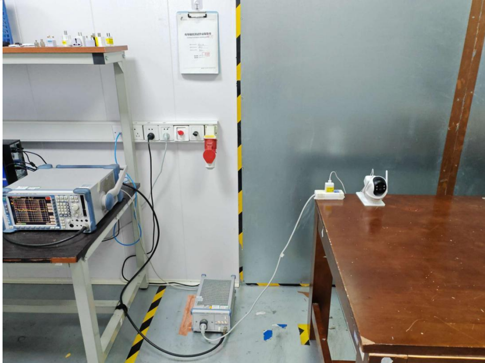
Conducted emissions at AC power line (150kHz-30MHz)
