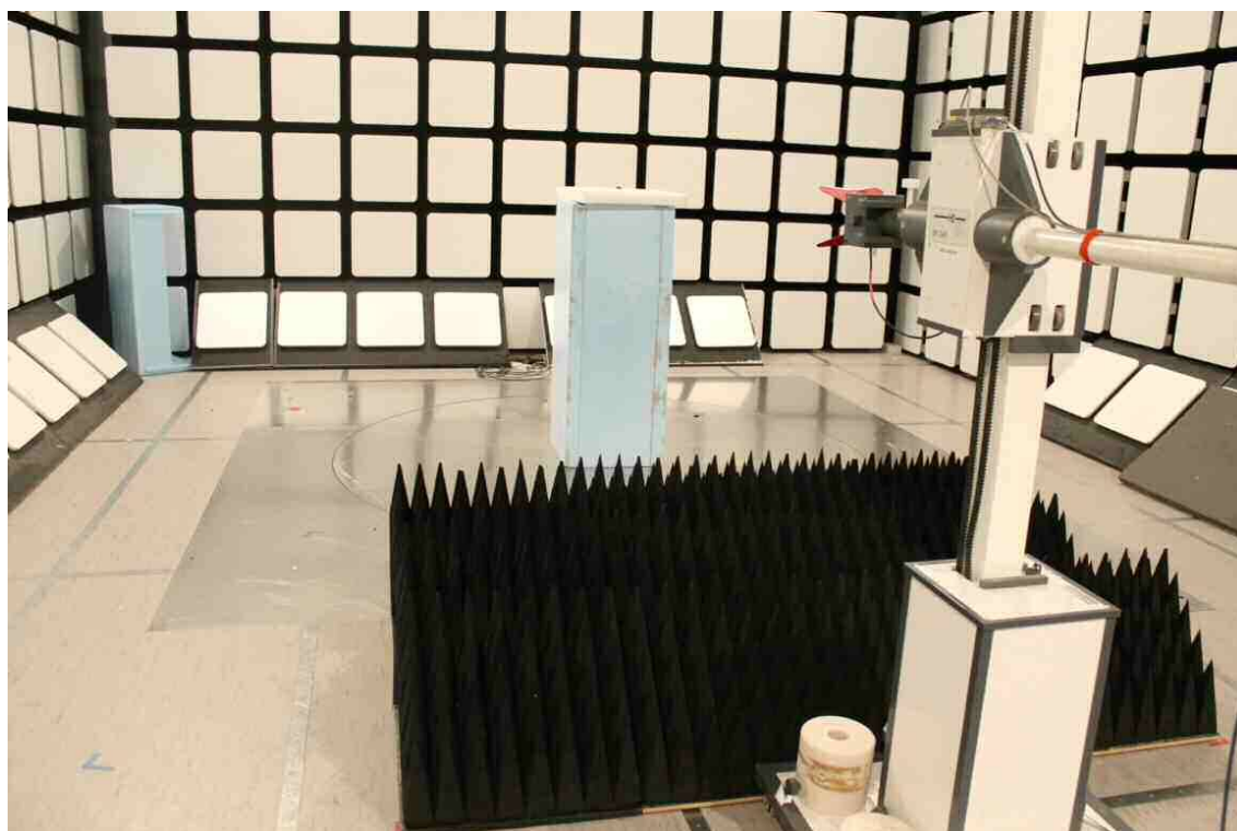
Photograph 2. Radiated Spurious Emissions 1 – 18 GHz
