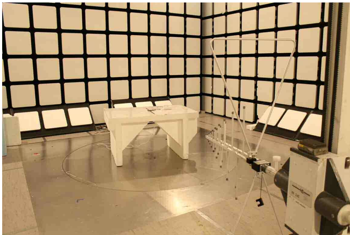
Photograph 1. Radiated Spurious Emissions 30 – 1000 MHz
