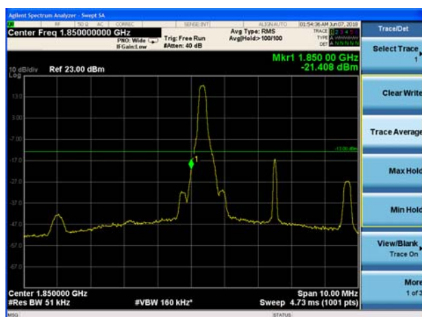
LTE Band 2 5MHz 16QAM 1RB CH-Low
