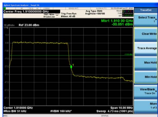
LTE Band 2 5MHz QPSK 100%RB CH-High
