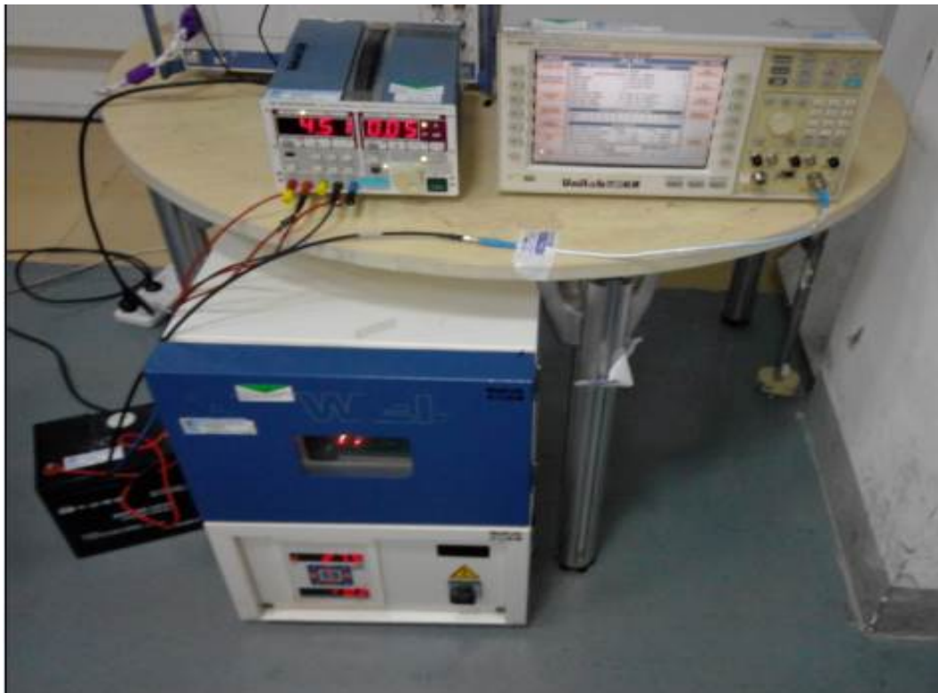
Frequency Stability Under Temperature & Voltage Variations Setup
