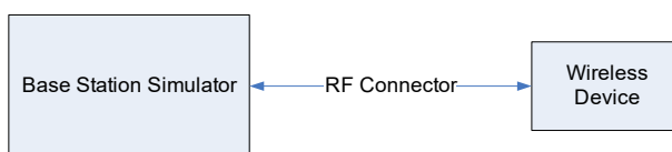
Figure 9-1 Power Measurement Setup
