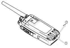
Note: Don't Attach / Remove the Battery if the transceiver turned on .
