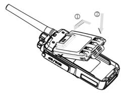
To remove the battery, Please turn the power off, then press the release latch to unlock the battery pull the battery away from the radio.
