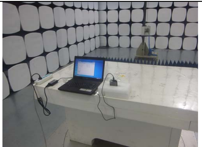
Radiated Spurious Emissions Test Setup Above 1GHz
