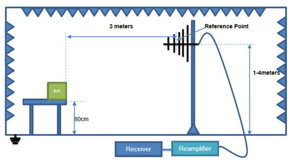
Radiation Test (30MHz - 1GHz)
