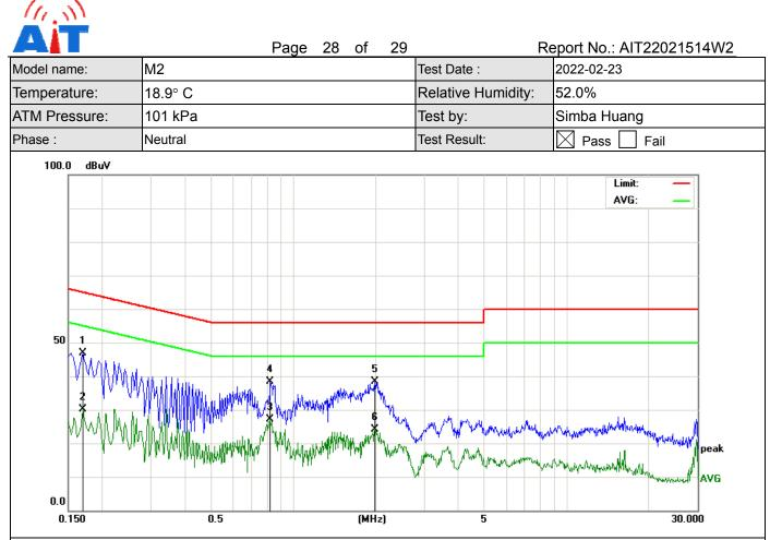
Remark: Factor = Antenna Factor + Cable Loss – Pre-amplifier. Measurement Result=Reading Level +Correct Factor; Over Limit= Measurement Result- Limit;
