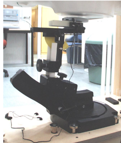
Fig.5.1.4.2. PDNNEM-4 in body position and spacer removed. Phone is on the polystyrene support and has stereo headset HDD-2 connected.
