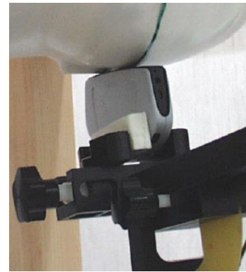
Fig. 5.1.3.2. Cheek position seen from backside of the phone. Polystyrene piece used as positioning support.
