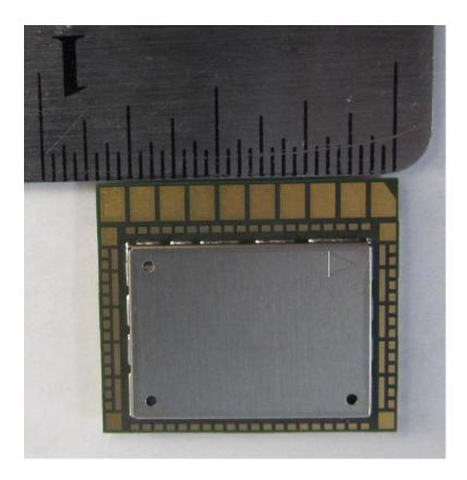
Figure 1-2 PWB side B with shields
