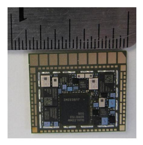
Figure 2-2 PWB side B without shields
