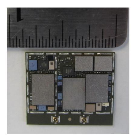
Figure 2-1 PWB side A without shields
