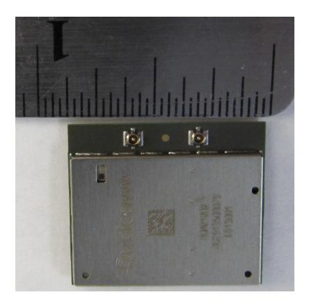
Figure 1-1 PWB side A with shields
