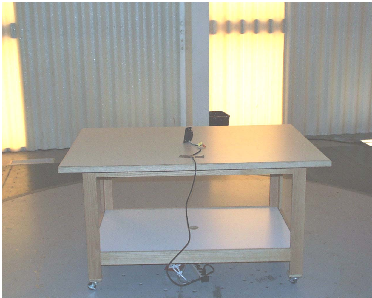
Photograph 2 - Back View Radiated Disturbance Worst Case Configuration
