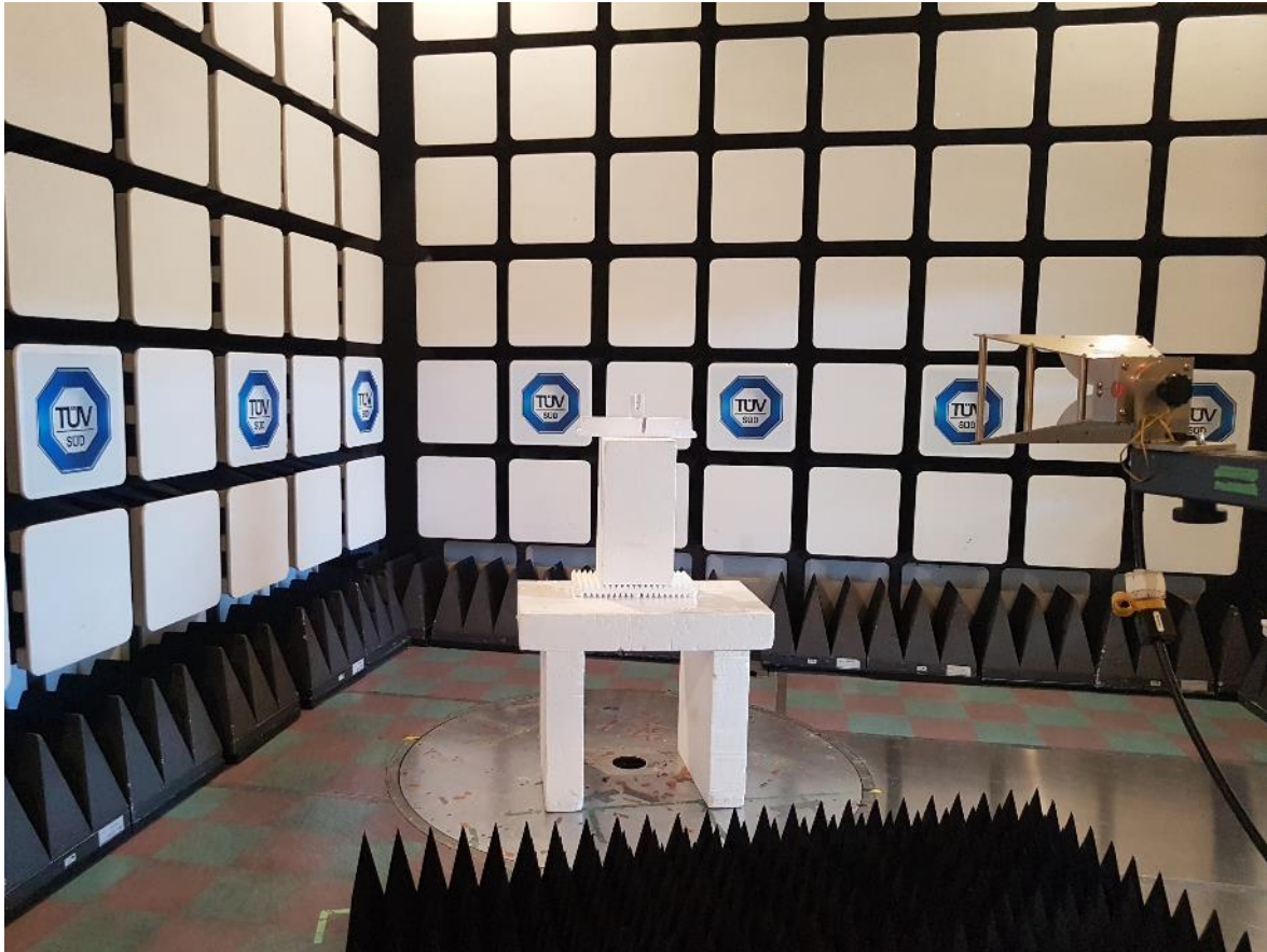
Figure 5 – Radiated Emissions Setup – Photo 4
