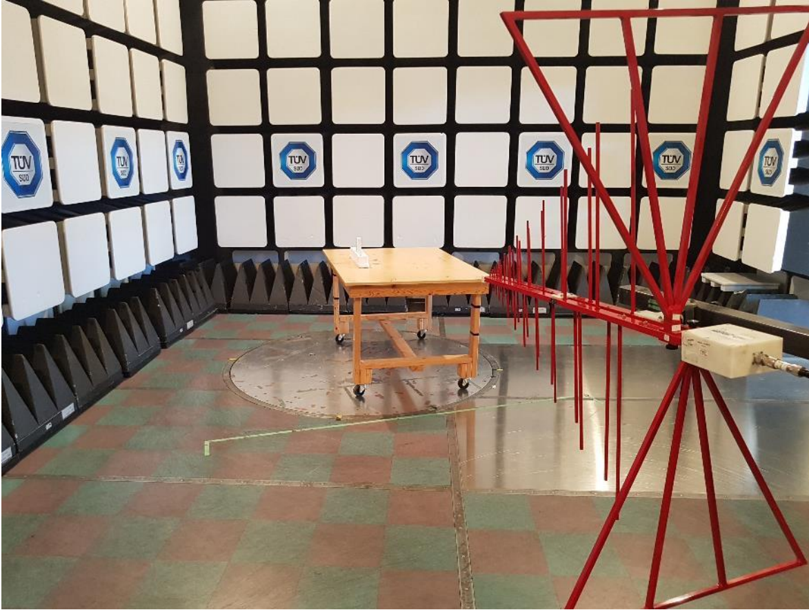
Figure 4 – Radiated Emissions Setup – Photo 3
