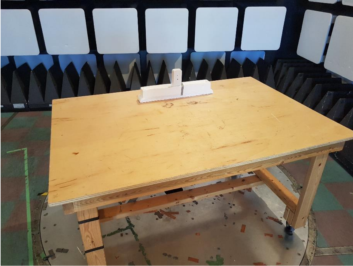
Figure 2 – Radiated Emissions Setup – Photo 1
