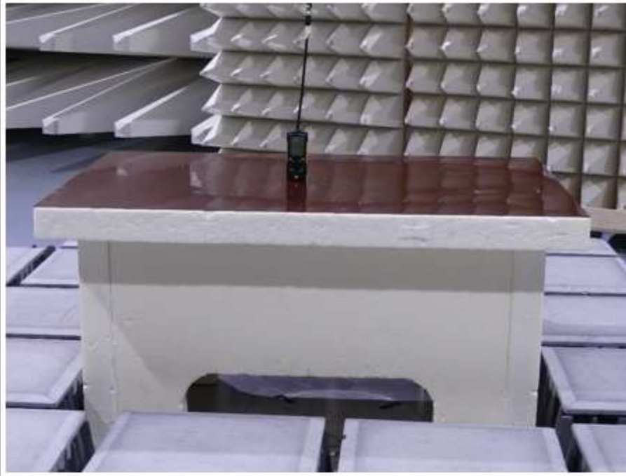
Test setup accumulator and Bluetooth, 1000-13000 MHz
