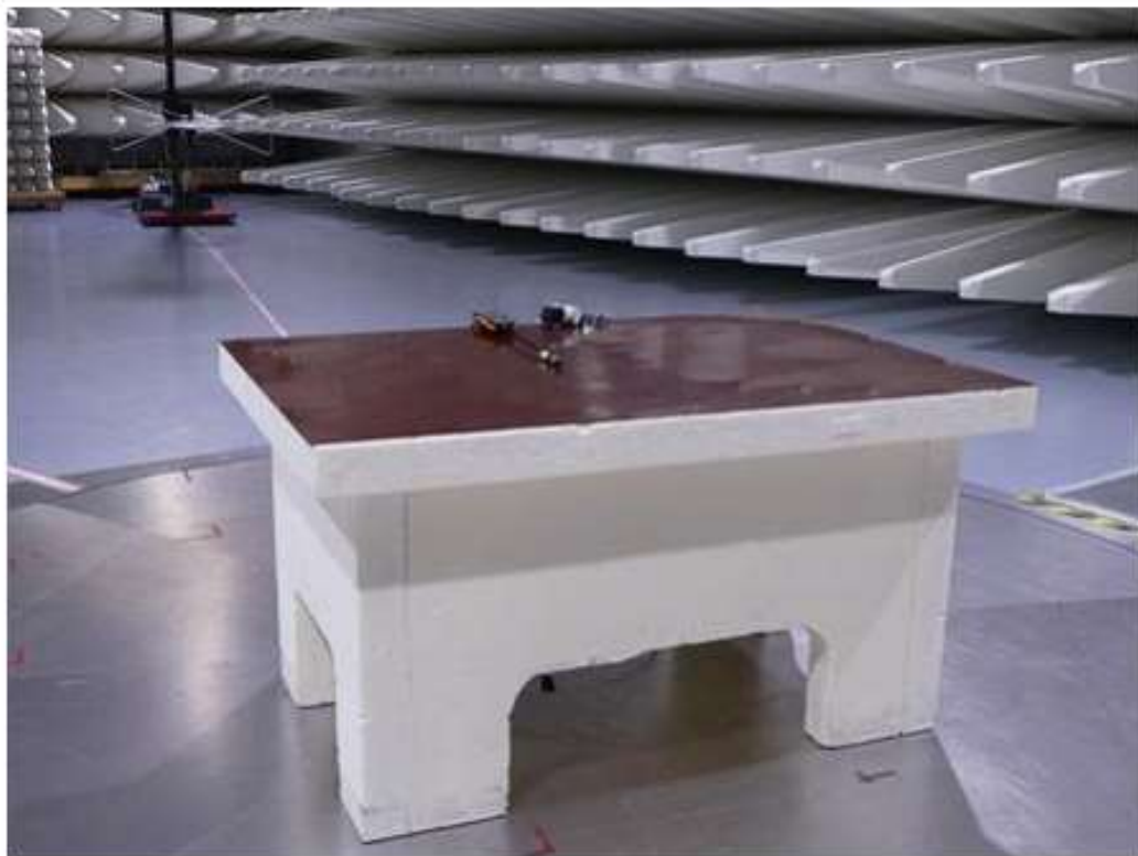
Setup 30 to 1000 MHz horizontal, charging mode (TESTO)
