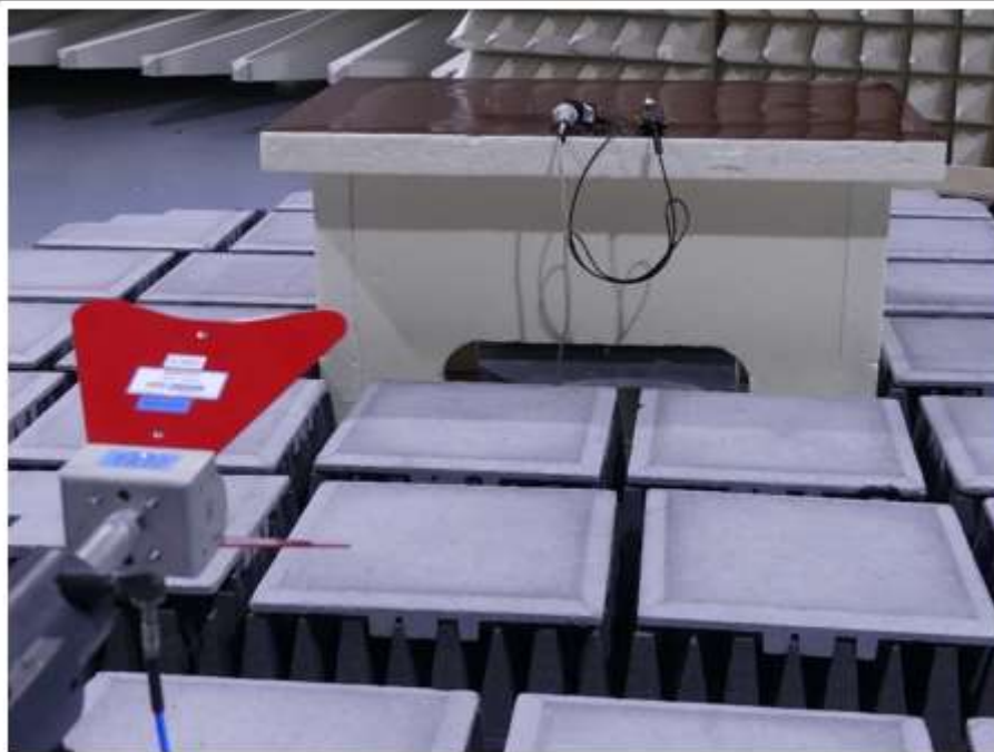
Test setup charging, 1000-13000 MHz (TESTO)
