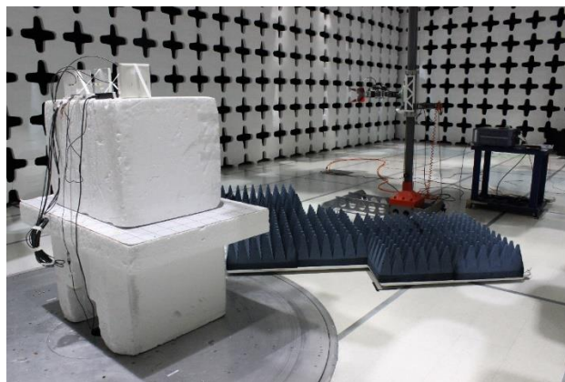
FCC RSE 1GHz to 18GHz – Rear View
