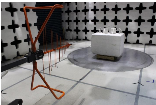
FCC RSE 30MHz to 1GHz – Front View
