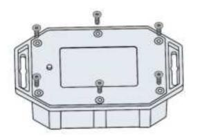
Step1: Remove the screws on the bottom of the device
