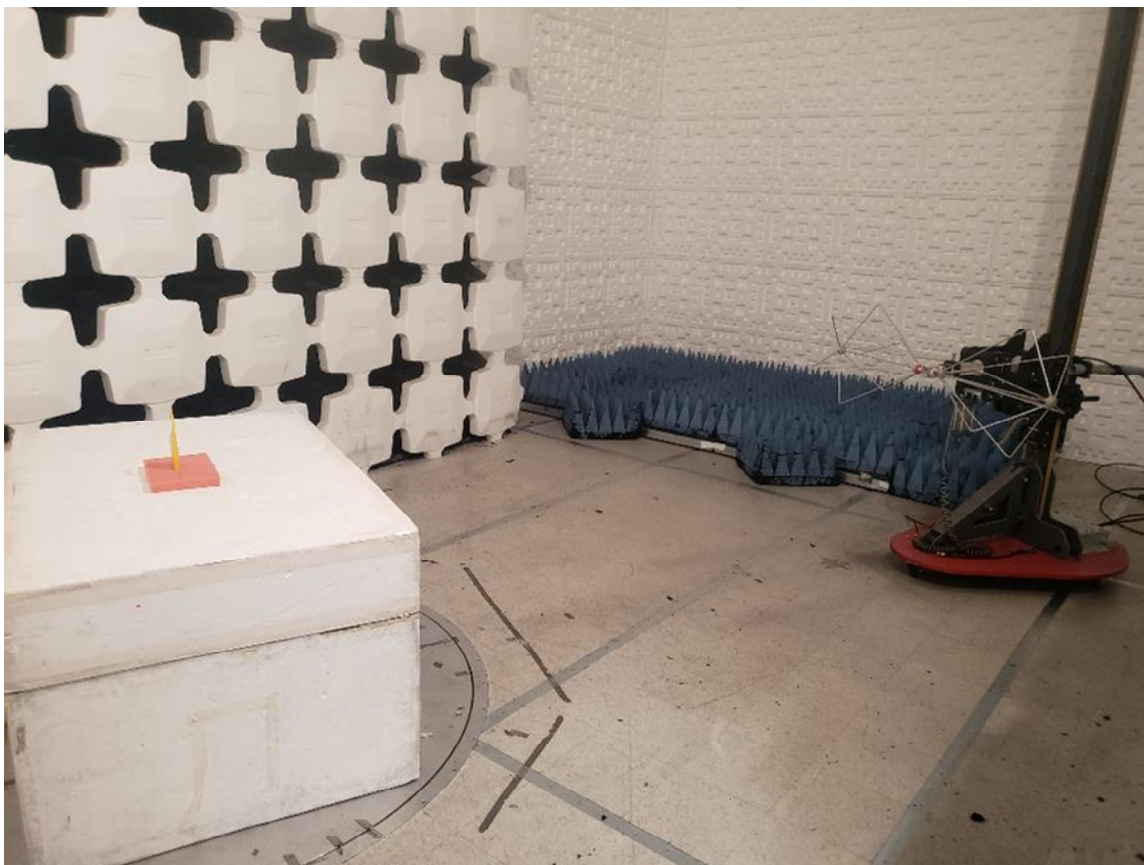
Figure 4. Radiated Emissions Test Setup (30 - 200 MHz)
