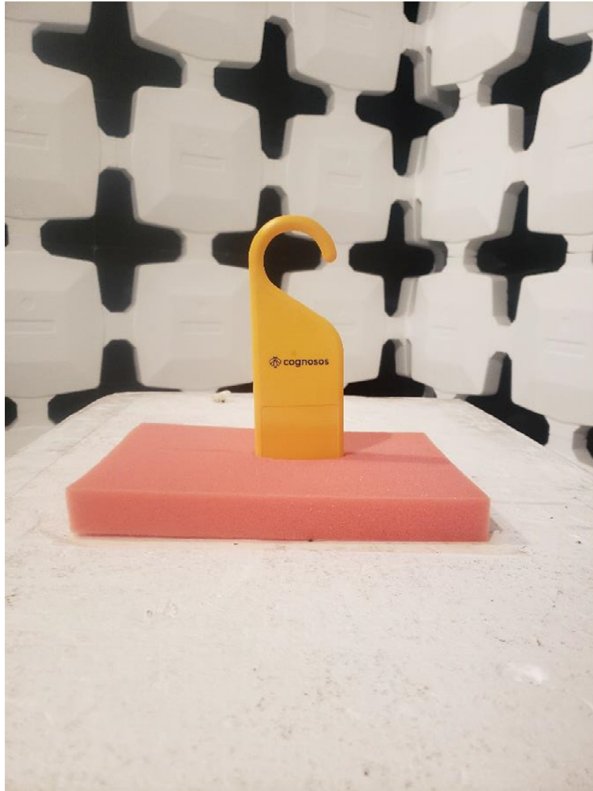
Figure 1. Radiated Emissions Test Setup, BT Radio
