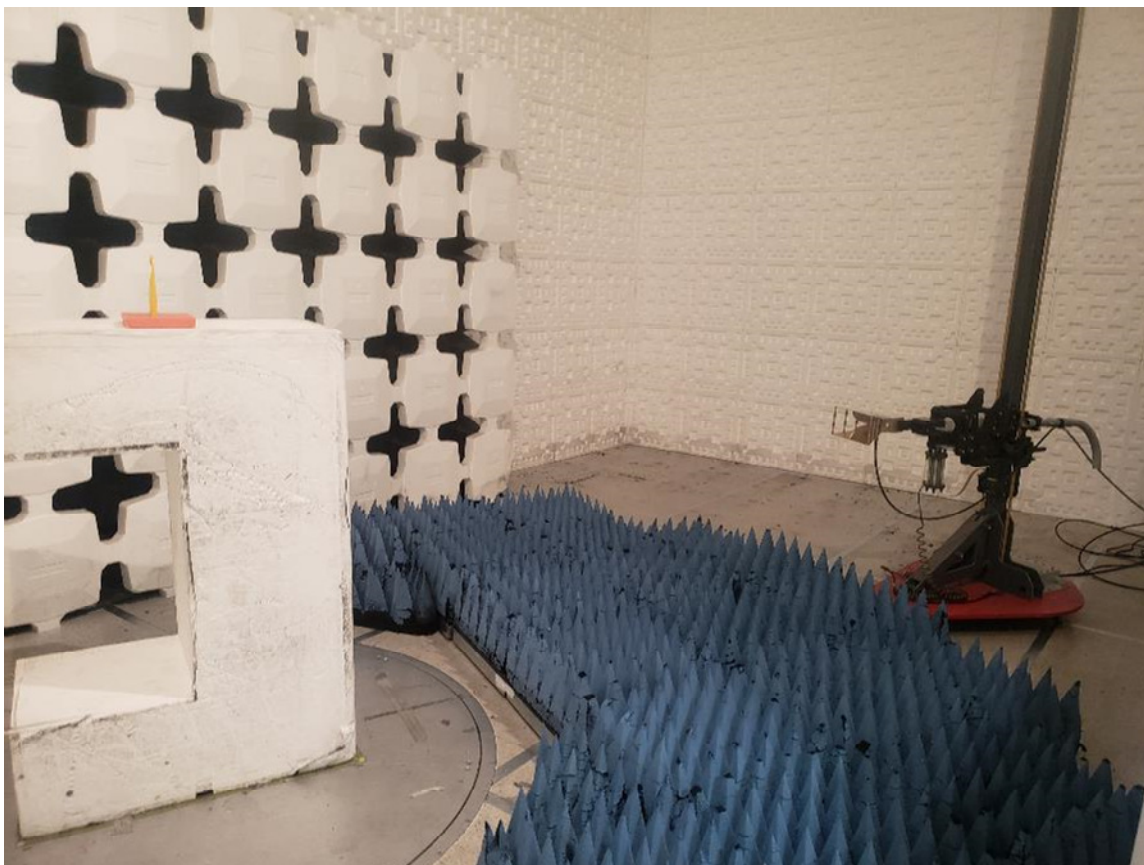
Figure 6. Radiated Emissions Test Setup (1 GHz – 6 GHz)
