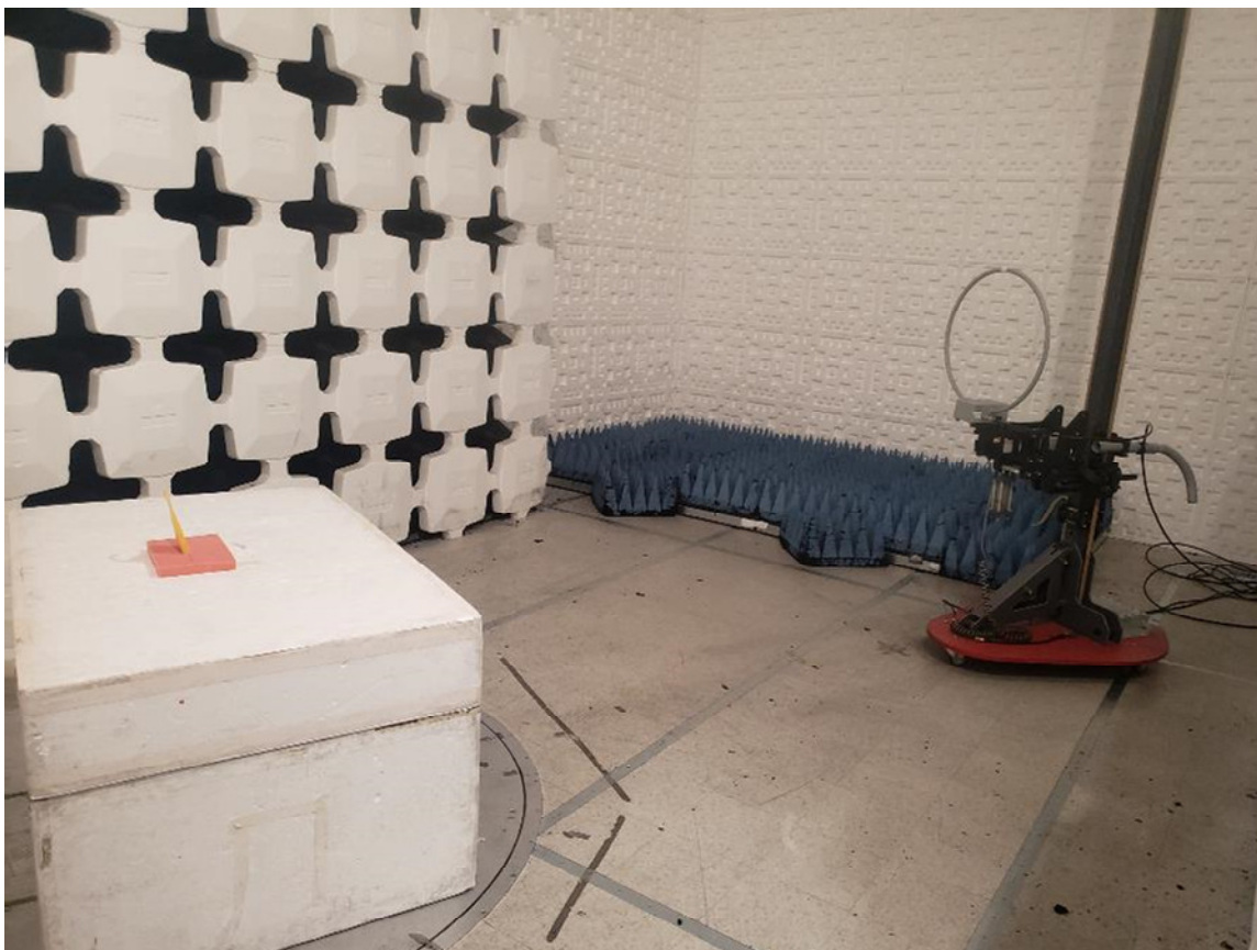
Figure 3. Radiated Emissions Test Setup (9 kHz - 30 MHz)
