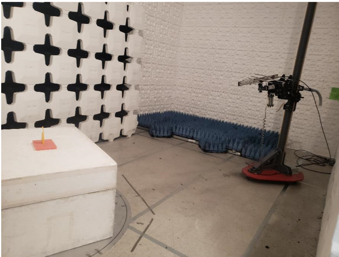
Figure 5. Radiated Emissions Test Setup (200 MHz - 1 GHz)
