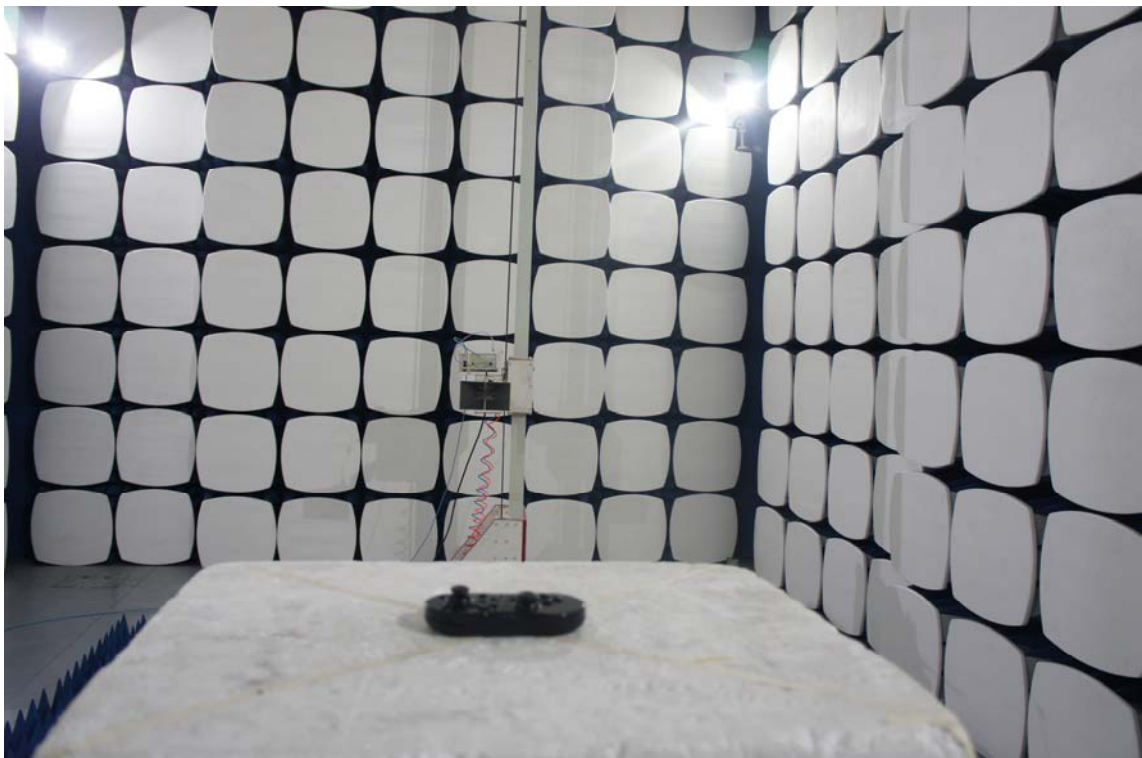
Radiated Setup photo (Above 1G)
