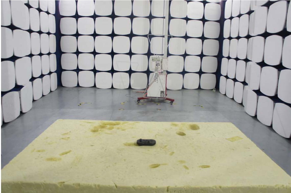
Radiated Setup photo (Below 1G)
