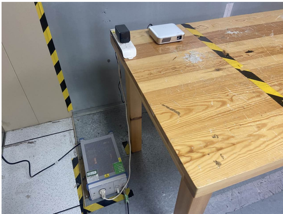
Conducted emission Test Setup
