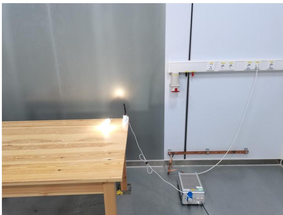
Fig. 4 Power line conducted emission setup photo
