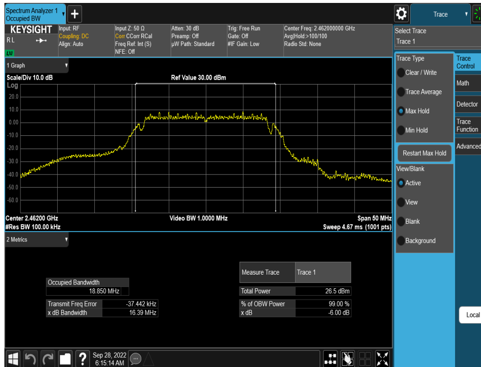
Plot 7-6. 6dB BW and 99% OBW Plot (802.11g – Ch. 11)
