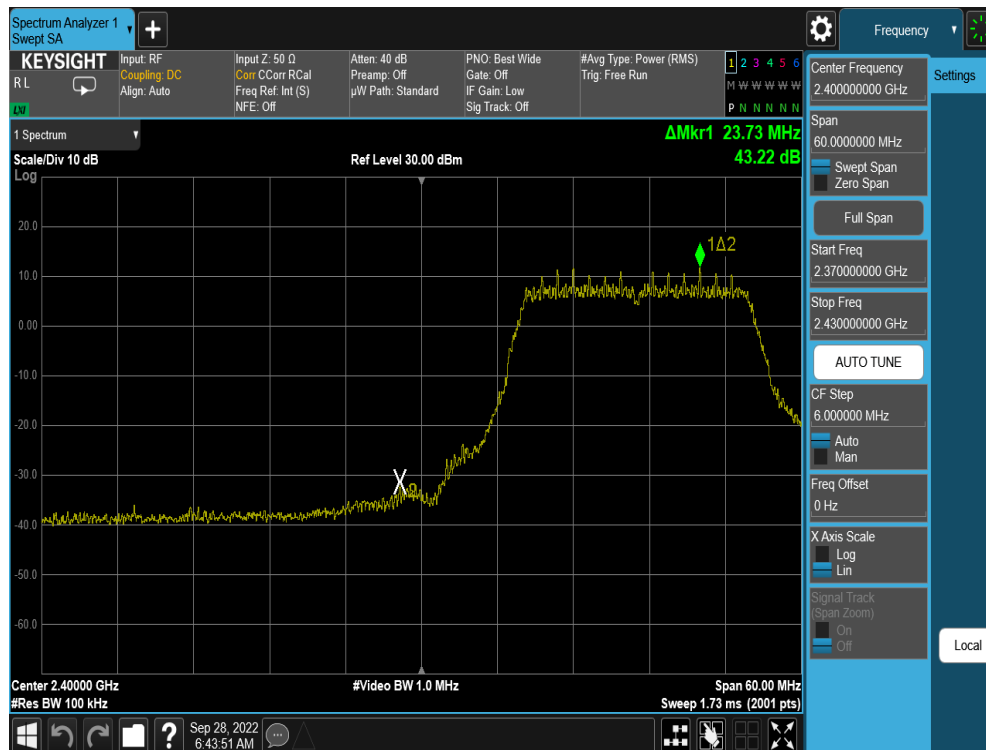
Plot 7-45. Band Edge Plot (802.11n MCS0 – Ch. 2)
