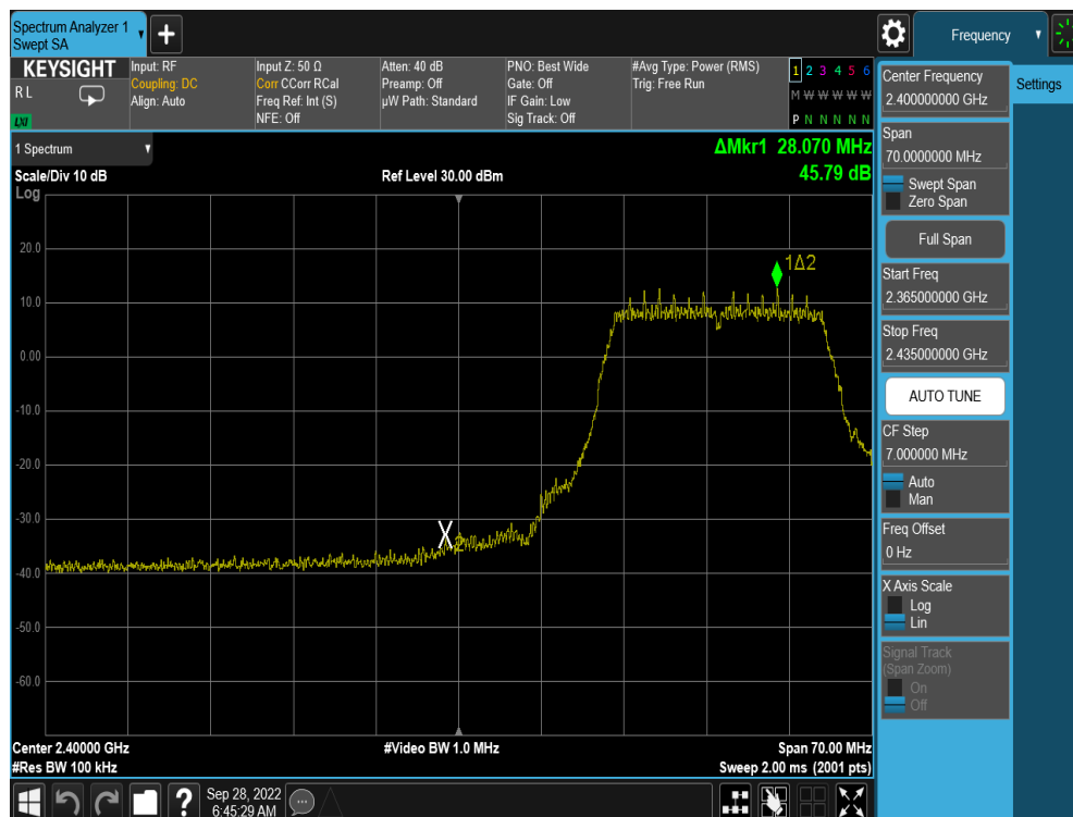
Plot 7-46. Band Edge Plot (802.11n MCS0 – Ch. 3)
