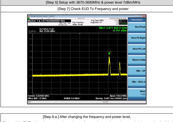
The module (EUT) discontinues operations, change frequencies, or change its operational power level within 10 seconds of receiving instructions from its associated CBSD. Test result is PASS.
