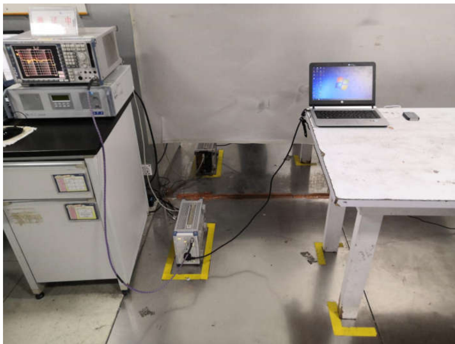
AC Conducted Emissions Test Setup
