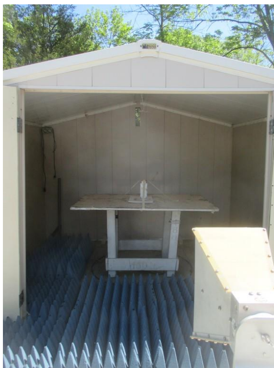
Figure 2 Radiated Emission Test Setup
