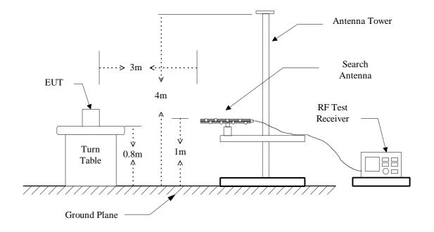
Figure 1 : Frequencies measured below 1 GHz configuration
