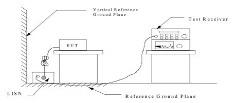
Figure 3 : Conducted emissions measurement configuration
