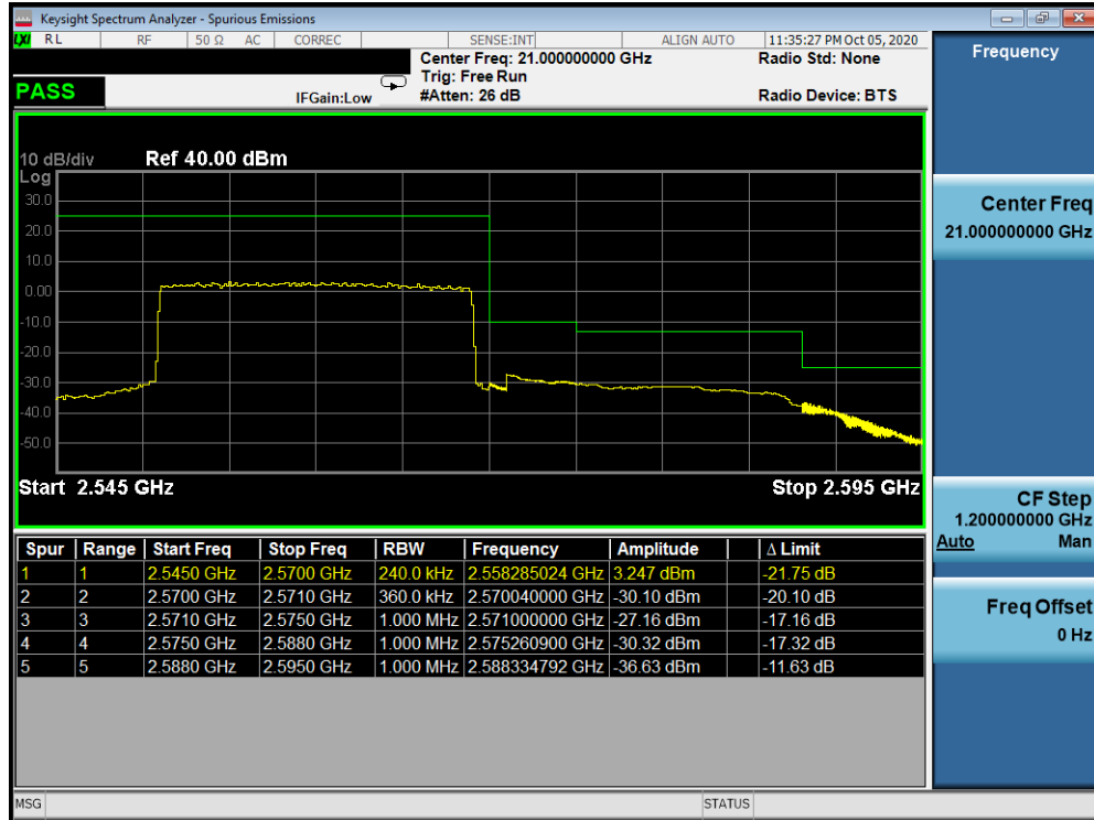
Plot 7-23. Upper ACP Plot (LTE Band 7 - 20MHz QPSK – Full RB Configuration)
