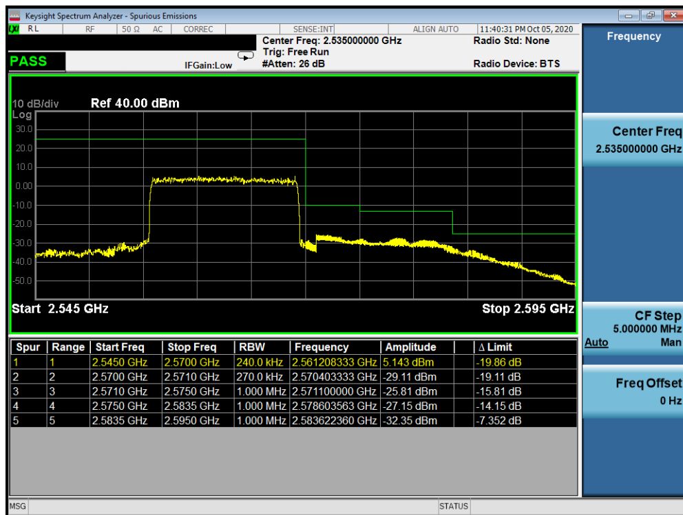
Plot 7-25. Upper ACP Plot (LTE Band 7 - 15MHz QPSK – Full RB Configuration)
