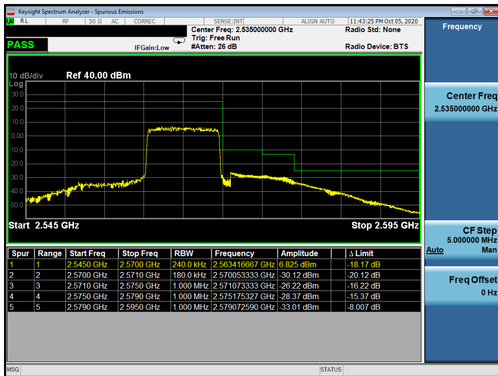
Plot 7-27. Upper ACP Plot (LTE Band 7 - 10MHz QPSK – Full RB Configuration)
