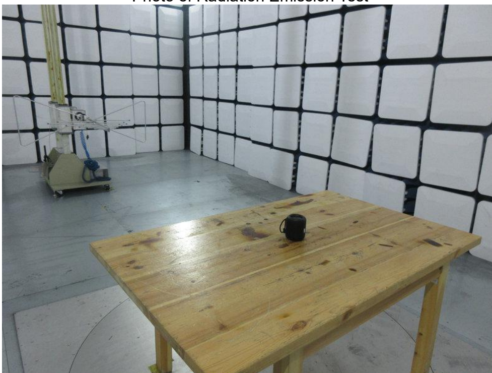
Photo of Radiation Emission Test
