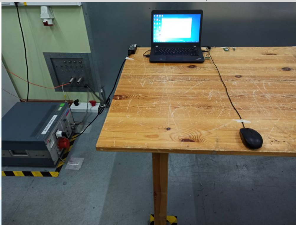
Conducted Emission Test Setup
