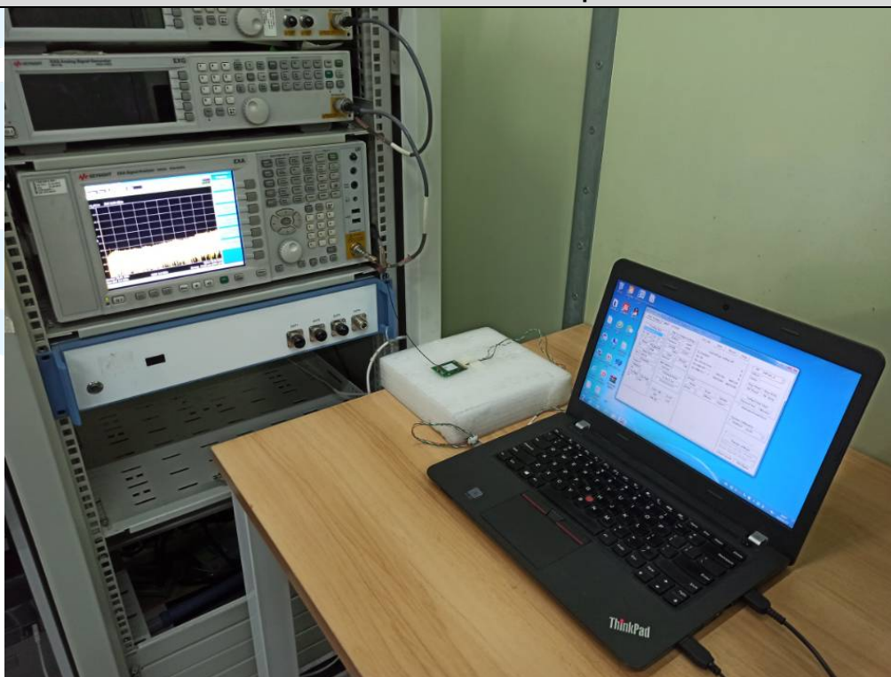
RF Conducted Test Setup
