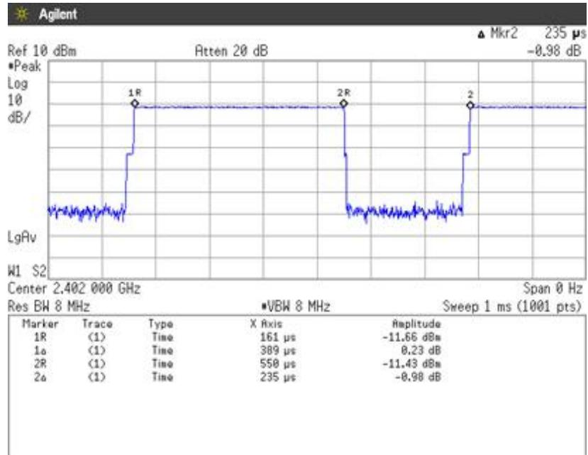
$$\text{Duty Cycle} = T_{\text{on}} / (T_{\text{on}} + T_{\text{off}}) = 389[\mu\text{s}] / (389[\mu\text{s}] + 235[\mu\text{s}]) = 62.34\%$$
