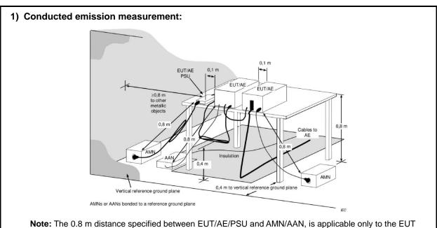
being measured. If the device is AE then it shall be >0.8 m.
