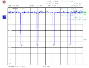
Duty cycle = 2.080 ms / 2.180 ms = 95.41% Duty Factor = 10 log(1/Duty cycle) = 0.20
