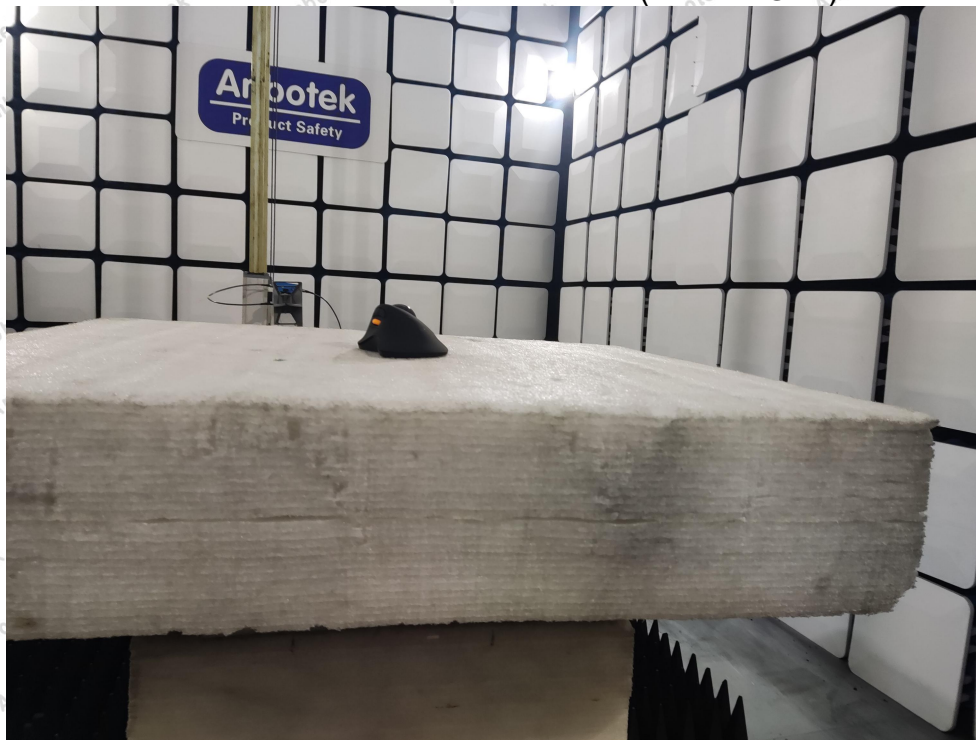
Photo of Radiation Emission Test (above 1GHz)
