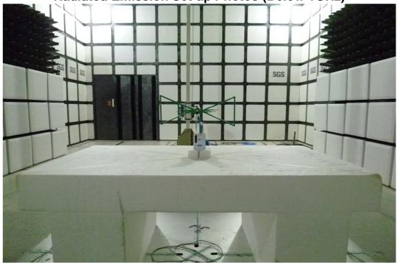
Radiated Emission Set up Photos (Above 1GHz)
