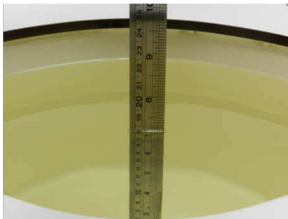
Fig 10.1 Photo of Liquid Height for Body SAR
