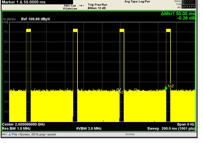
Time Between Pulses = 50 ms Total On Time = 4.86 ms Total Duty Cycle = 4.86 ms / 50.00 ms = 9.72% The Maximum Peak to Average Ratio of -20 dB can be used.
