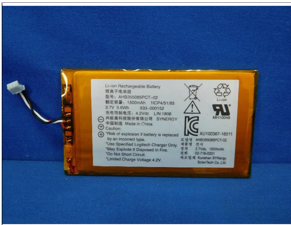
Battery 2: (Model: AHB355085PCT-02 or 533-000152)
