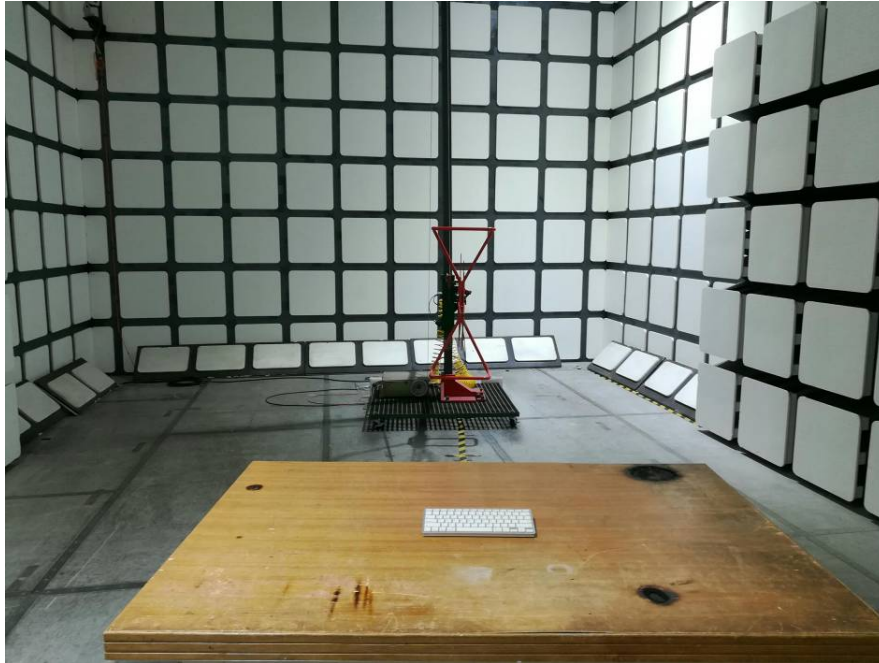
Radiated Emissions View (Below 1 GHz)
