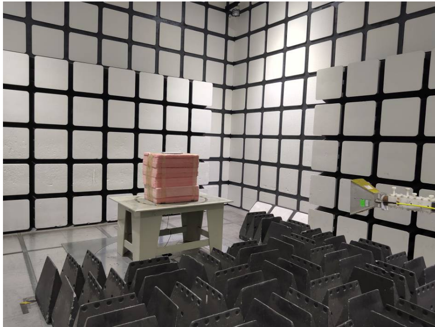
Radiated Emissions View (Above 1 GHz)
