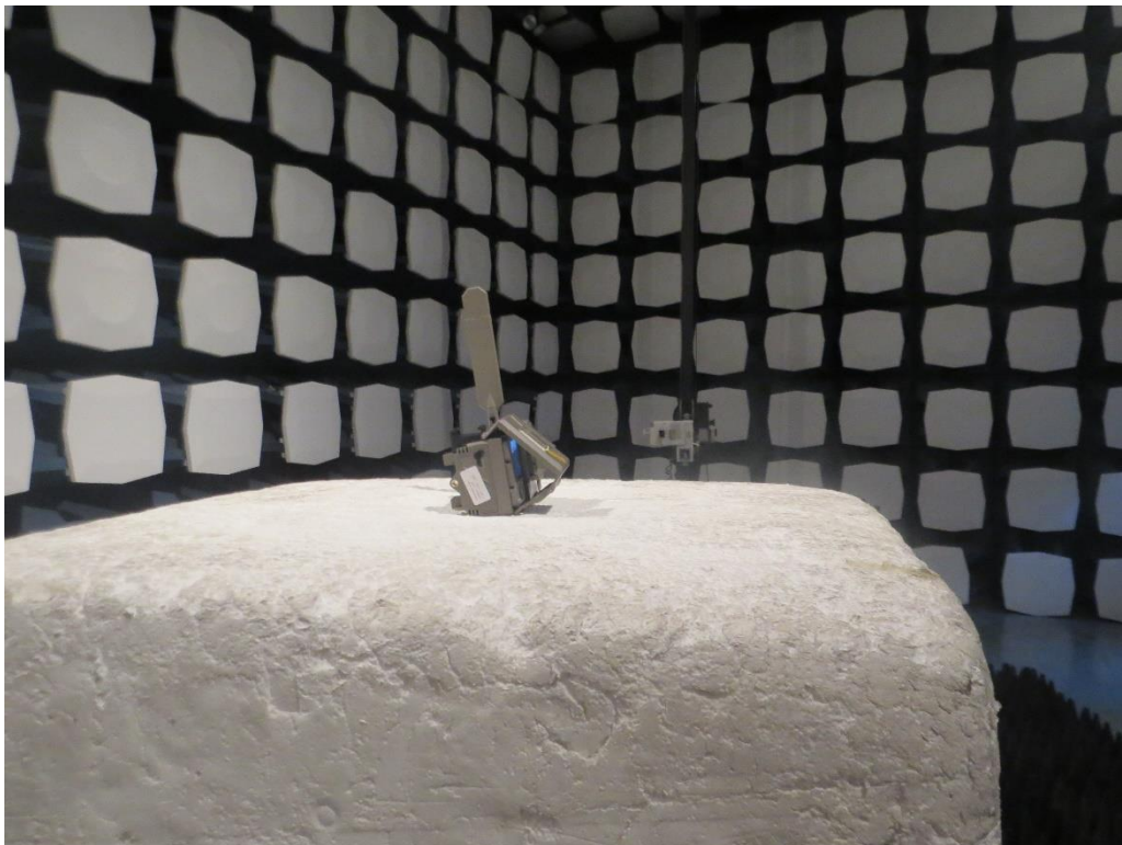
Picture 1: Radiated Spurious Emissions Test setup
