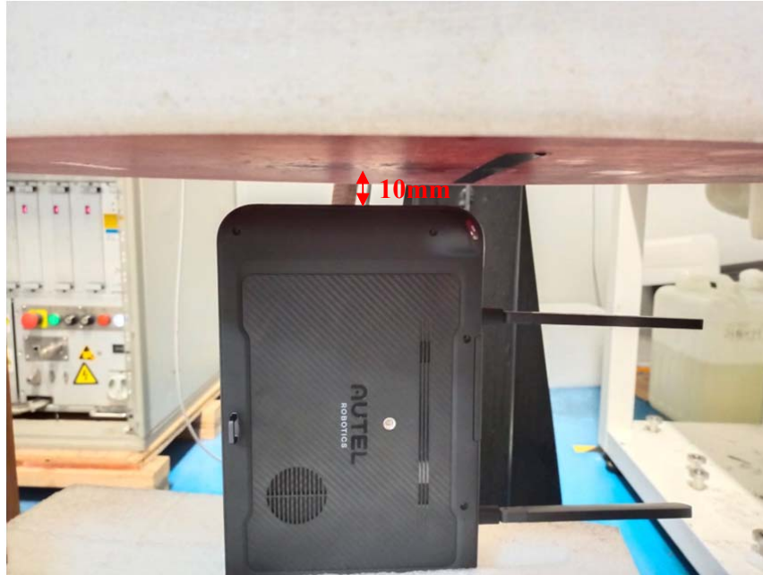
Close to Body RighSetup Photo(10mm)
