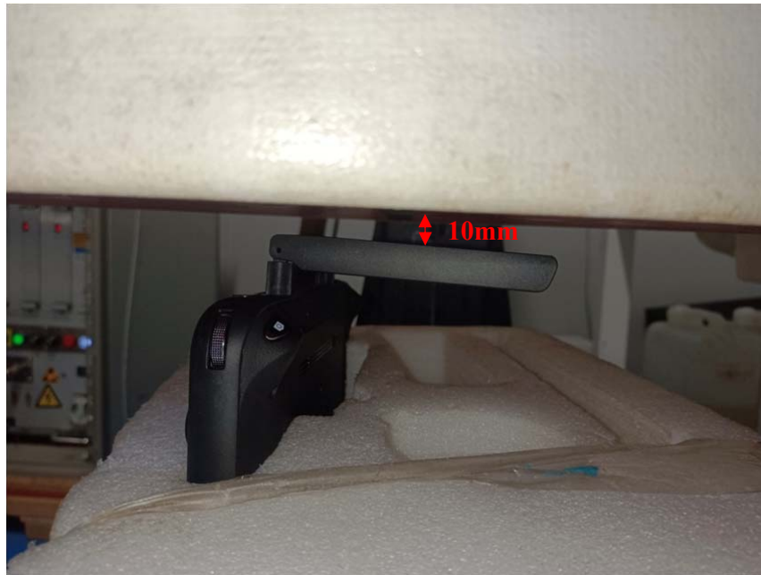
Close to Body TopSetup Photo(10mm)
