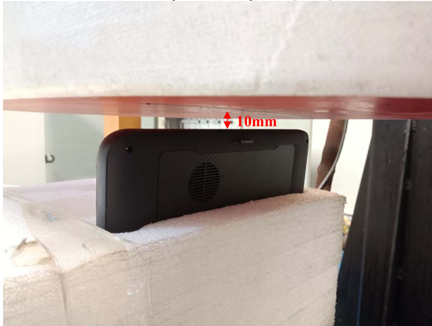
Close to Body Bottom Setup Photo(10mm)
