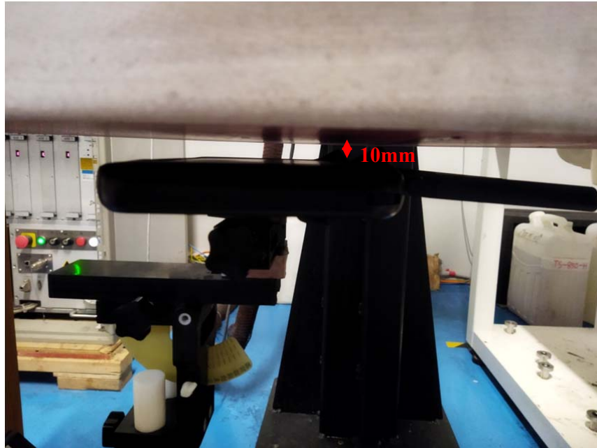
Close to Body Back Setup Photo(10mm)
