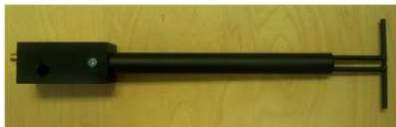
Figure 1 – MVG COMOSAR Validation Dipole
