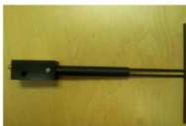
Figure 1 – MVG COMOSAR Validation Dipole
