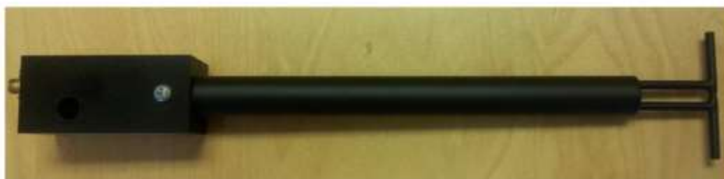
Figure 1 – MVG COMOSAR Validation Dipole
