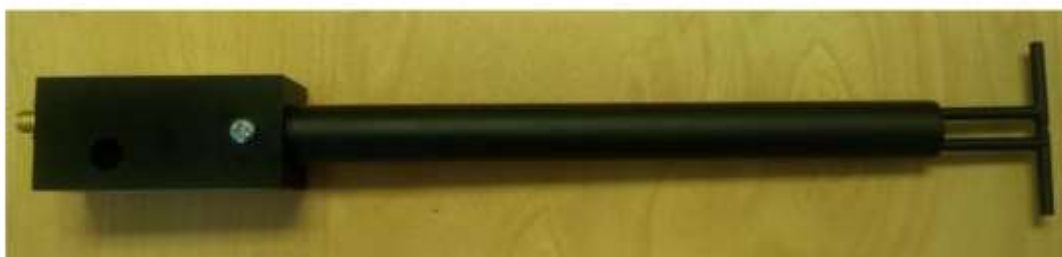
Figure 1 – MVG COMOSAR Validation Dipole
