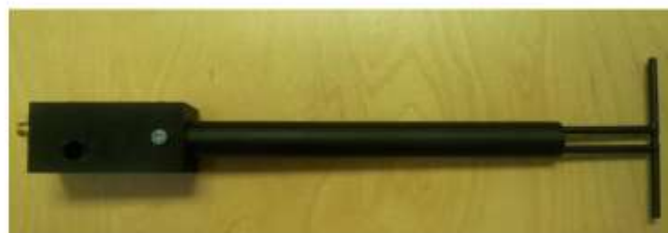
Figure 1 – MVG COMOSAR Validation Dipole
